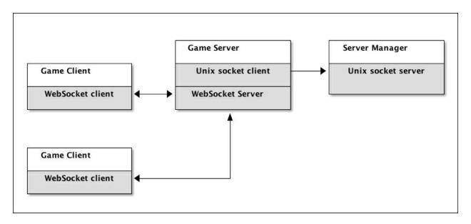
In this diagram, we can see the **Server Manager** application on the right. It communicates via Unix sockets with a single instance of **Game Server**. This instance of **Game Server** has two clients connected to it via WebSockets.
